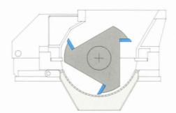
Entrance to the cutting chamber is offset for tangential feed of material, resulting in virtually no flyback. Close rotor to screen clearance prevents blockage and material build-up in chamber.
