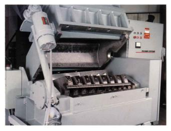
Split chamber design with power assisted tilting hopper provides easy access for knife adjustment and cleanout. Cutting chamber and screen cradle are interlocked for safety.
