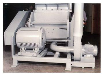
Heavy duty motor and long lasting, wear resistant evacuation blower can be integrally mounted at the base of the machine, as shown.
