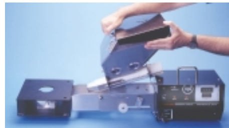
MCF Hopper being removed
