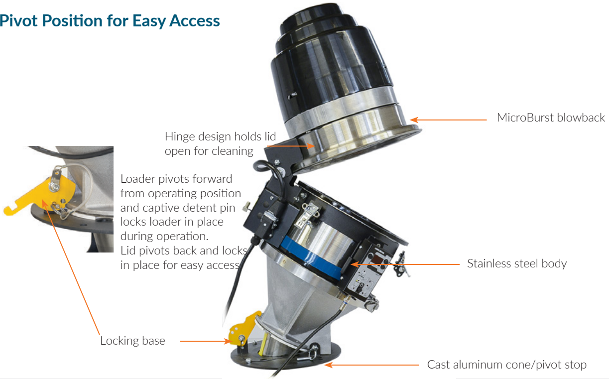
Loader pivots forward from operating position and captive detent pin locks loader in place during operation. Lid pivots back and locks in place for easy access.
