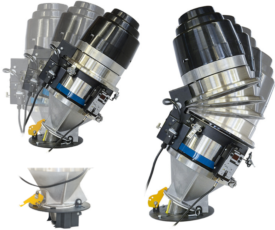
Loader pivots forward from operating position and captive detent pin locks loader in place during operation. Lid pivots back and locks in place for easy access.
